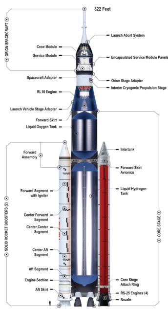
This cutaway illustration identifies the major elements of the SLS and Orion stack. The SLS portion consists of, from the ground up: twin solid rocket boosters with major components labeled, RS-25 liquid-fuel engines, central core stage with propellant tanks and flight computers, launch vehicle stage adapter, ICPS, and Orion stage adapter. Orion is atop SLS. A 6-ft. figure is shown for comparison in the lower left.
