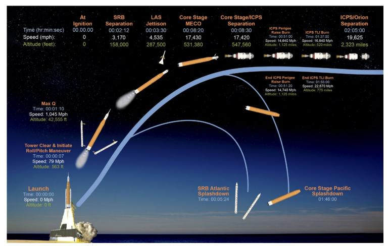
Major events of the Artemis I flight, including solid rocket booster jettison, core stage and launch vehicle stage adapter separation, and ICPS and Orion stage adapter separation from Orion. Following separation with Orion, CubeSat payloads will be released into deep space.
