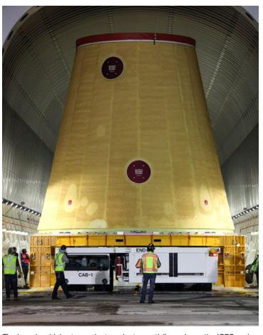
The launch vehicle stage adapter adapter partially encloses the ICPS and contains the pyrotechnic system to separate itself and the core stage from the ICPS and Orion.
