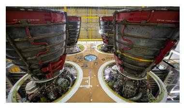
The Artemis I RS-25 engines installed in the core stage during assembly at NASA's Michoud Assembly Facility in New Orleans.
