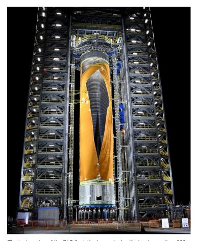
The test version of the SLS liquid hydrogen tank withstood more than 260 percent of expected flight loads over five hours before it buckled, then ruptured, giving engineers real-world data to reinforce computer models.
