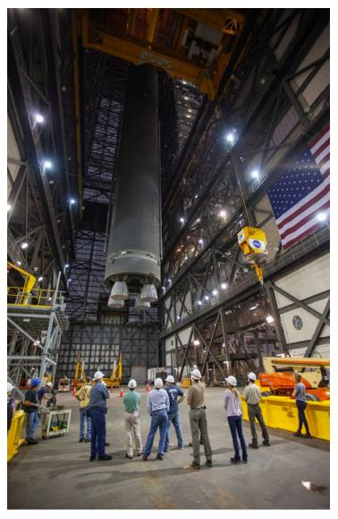
Engineers and technicians at Kennedy used the 212-ft. (65 m) pathfinder core stage simulator to practice lifts and moves in the Vehicle Assembly Building.
