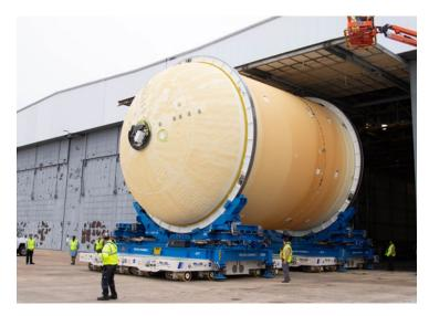
The liquid oxygen tank being manufactured for the Artemis I flight at Michoud.
