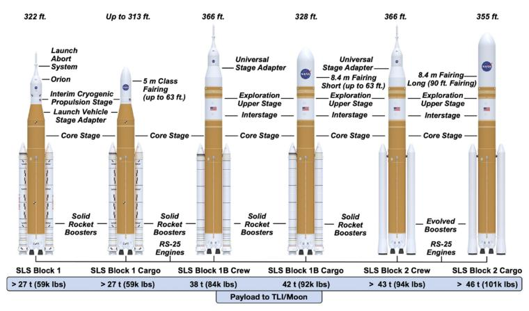
SLS Block 1 with an uncrewed Orion will launch the Artemis I mission. Following the first three Artemis missions, SLS will evolve to a more powerful Block 1B configuration with a new Exploration Upper Stage replacing the ICPS. The ultimate variant, Block 2, will incorporate evolved boosters to increase payload mass to TLI to at least 101,000 lbs. (46 t).
