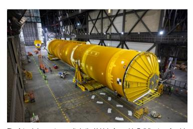
The Artemis I core stage waits in the Vehicle Assembly Building transfer aisle before stacking on the mobile launcher.
