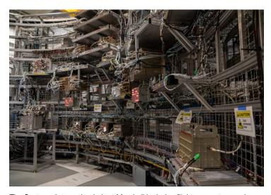
The Systems Integration Lab at Marshall includes flight computers and avionics functionally identical to the core stage avionics to test all systems prior to flight.
