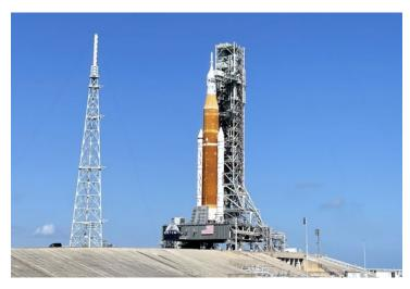
Stacked Artemis I rocket, consisting of SLS and Orion, on the mobile launcher.
