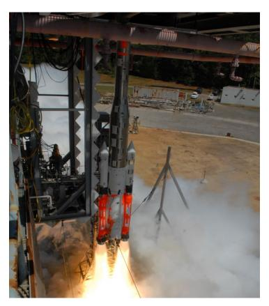
A five-percent scale model of SLS undergoes acoustic testing in 2014 at Marshall.
