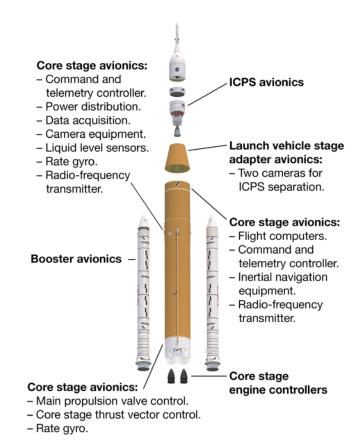
Avionics throughout the elements of SLS monitor the rocket's health and control the flight.
