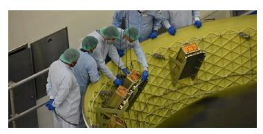
The Artemis I Orion stage adapter with mounting brackets for secondary payloads.
