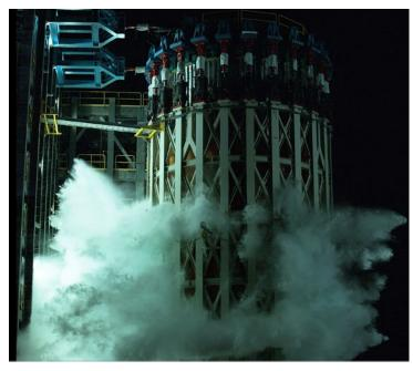
Hydraulic cylinders applied millions of pounds of force to the liquid oxygen tank test article, completing 20 tests until it failed, providing engineers with valuable data on the tank's structural capabilities.
