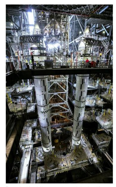
The completed Artemis I boosters are shown stacked on the mobile launcher in the Vehicle Assembly Building at Kennedy Space Center before integrating the other elements of SLS and Orion.
