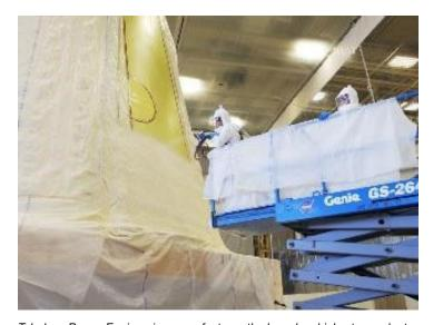
Teledyne Brown Engineering manufactures the launch vehicle stage adapter at Marshall, where technicians manually apply spray-on insulation, which turns orange in sunlight.
