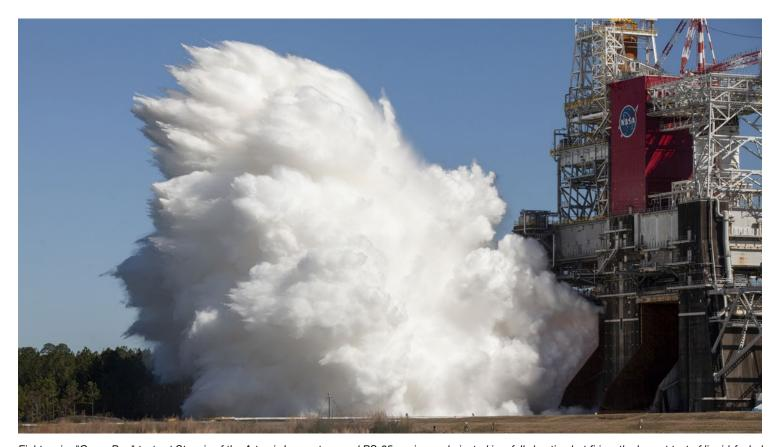
Eight major "Green Run" tests at Stennis of the Artemis I core stage and RS-25 engines culminated in a full-duration hot firing, the largest test of liquid-fueled engines since the Apollo Program.
