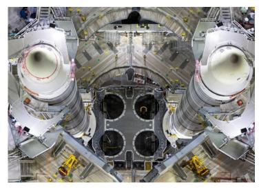
Birds-eye view of the Artemis I solid rocket boosters, the first element to be stacked on the mobile launcher in the Vehicle Assembly Building, awaiting the core stage.
