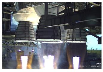
The Artemis I RS-25 liquid fuel engines operated successfully as part of the core stage Green Run hot fire test at Stennis in early 2021.
