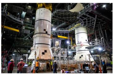
Artemis I booster aft assemblies ready for stacking in Kennedy Vehicle Assembly Building.
