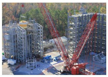
The Integrated Structural Test at Marshall included applying loads 40 percent greater than expected during launch to test versions of the launch vehicle stage adapter, frangible joint assembly, ICPS, Orion stage adapter, and a mass simulator for Orion.
