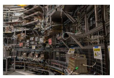
The Systems Integration Lab/Systems Integration Test Facility at Marshall is a full-scale mockup of flight-like avionics systems for the solid rocket boosters and core stage where engineers can test hardware and software integration prior to manufacture and flight.
