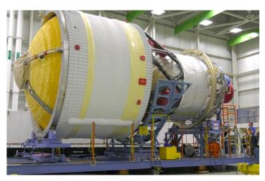
The ICPS is a single-engine liquid hydrogen/liquid oxygen stage based on the Delta Cryogenic Second Stage from ULA that produces 24,750 lbs. (110 t) of thrust and performs the TLI burn to send Orion toward the Moon.
