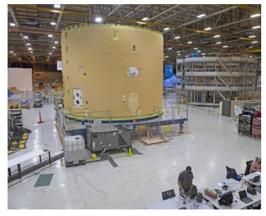
The SLS Artemis I intertank at Michoud, prior to integration between the propellant tanks, has forward attach points for the two solid rocket boosters.
