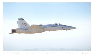
In 2013, NASA conducted a series of F/A-18 research flights to test SLS prototype software, including the previously adaptive augmenting control component. Adaptive augmenting contol benefits total attitude control and increases flight control system performance when excessive tracking error is present and decreases responsiveness to undesirable frequency content. It expands the envelope under which the flight control system is capable of safely flying the vehicle.
