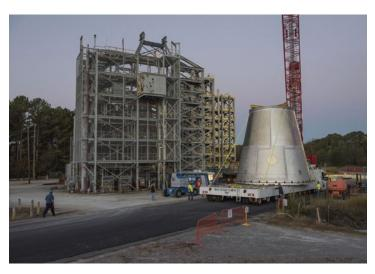
The launch vehicle stage adapter structural test article for the Integrated Structural Test was manufactured and tested at Marshall.
