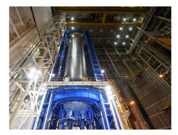
The Vertical Assembly Center at Michoud is one of the world's largest welding tools and is used to execute vertical friction-stir welds of the SLS core stage liquid hydrogen tank.
