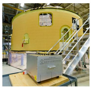
The core stage forward skirt contains the flight computers for the Block 1 SLS rocket.
