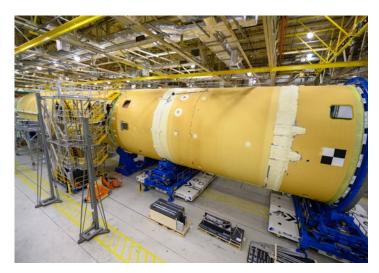
Connecting feedlines and other external components to the fully assembled Artemis I core stage at Michoud.
