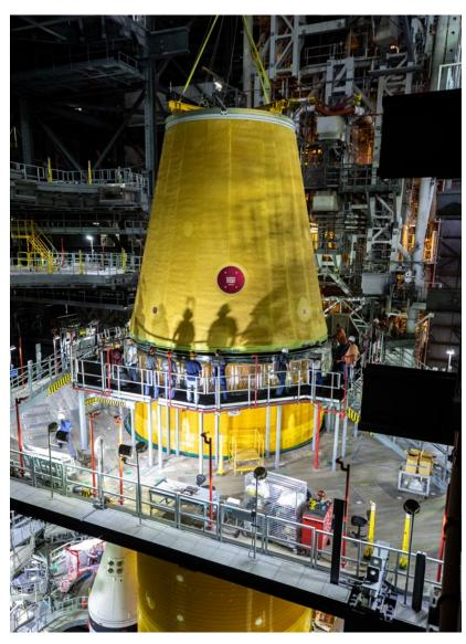
Teledyne Brown Engineering is the lead contractor for the launch vehicle stage adapter that has a pneumatically activated frangible joint that separates it and the core stage from the ICPS, Orion stage adapter, and Orion during flight.
