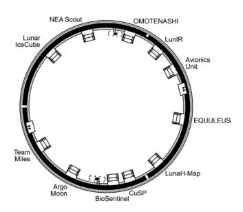
Payload berth locations on the Orion stage adapter.
