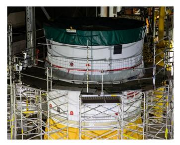
The ring-shaped Orion stage adapter is filled with 10 shoebox-sized CubeSats that will deploy when the ICPS separates from Orion on its way to the Moon.
