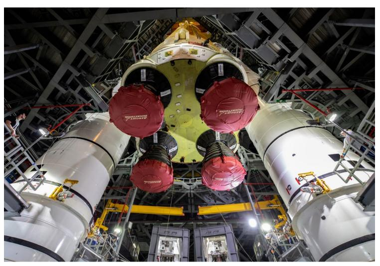
The Artemis I core stage is lowered between the SLS solid rocket boosters in the Vehicle Assembly Building. The SLS design uses a proven propulsion system of solid rocket boosters and liquid-fuel RS-25 engines to launch more payload to the Moon than any rocket since the Saturn V.
