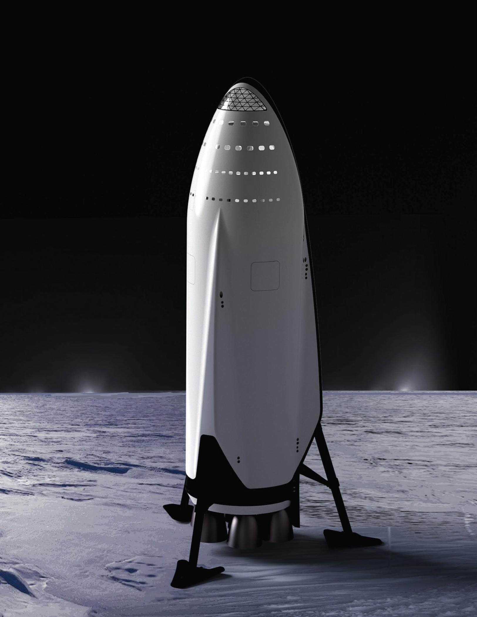
draw any connections. The launch height of the ITS is 122 meters, compared to the 111 meters of the Saturn V. Additionally, the Saturn V was designed as a single use vehicle, delivering it's payload into orbit using an expendable three stage setup, meaning that after each use the hardware is simply dropped into the ocean. On the other hand, the Interplanetary Transportation System is a two stage vehicle and is designed to be fully reusable.
