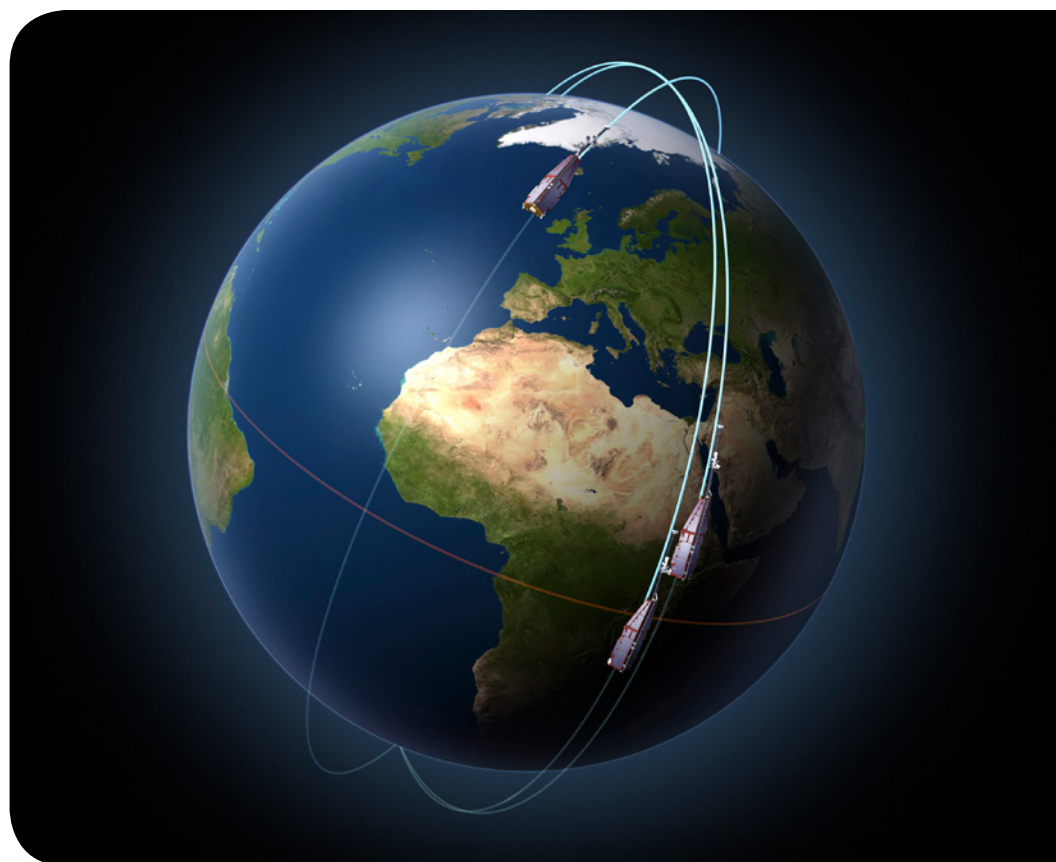
The ESA's three identical Swarm satellites were launched together. Two satellites orbit almost side-by-side at the same altitude. The third satellite is in a higher orbit and at a slightly different inclination.
