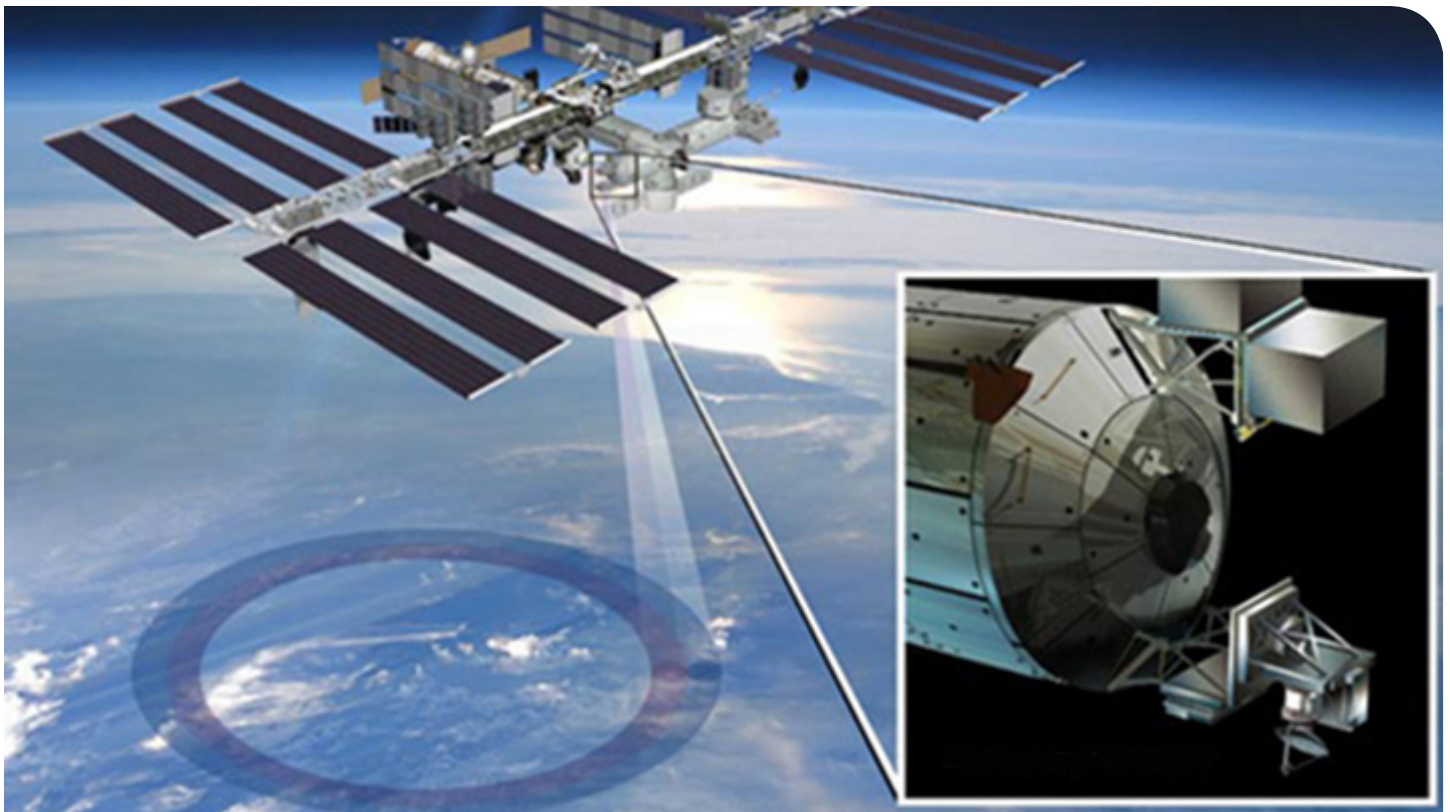
Artist's rendering of NASA's ISS-RapidScat instrument (inset), which will launch to the International Space Station in 2014 to measure ocean surface wind speed and direction and help improve weather forecasts, including hurricane monitoring. It will be installed on the end of the station's Columbus laboratory.
