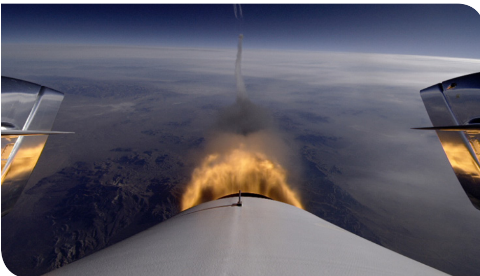
Tail-cam view of the hybrid engine burning during a test flight of SpaceShipTwo which saw the vehicle ascend to 71,000 feet over the Mojave Desert. Photo: Virgin Galactic
