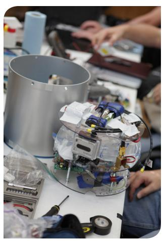
UP Aerospace personnel attached each student team's experiments to Plexiglas shelves that would fit in aluminum payload canisters. Photo: NM Student Launch Program
