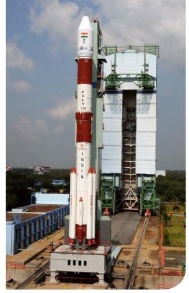
The PSLV-C25 rocket (above) undergoing launch rehearsal with the Moible Service Tower retracted. The MOM spacecraft (below) is being integrated to the fourth stage of its rocket. *Photos: ISRO*
