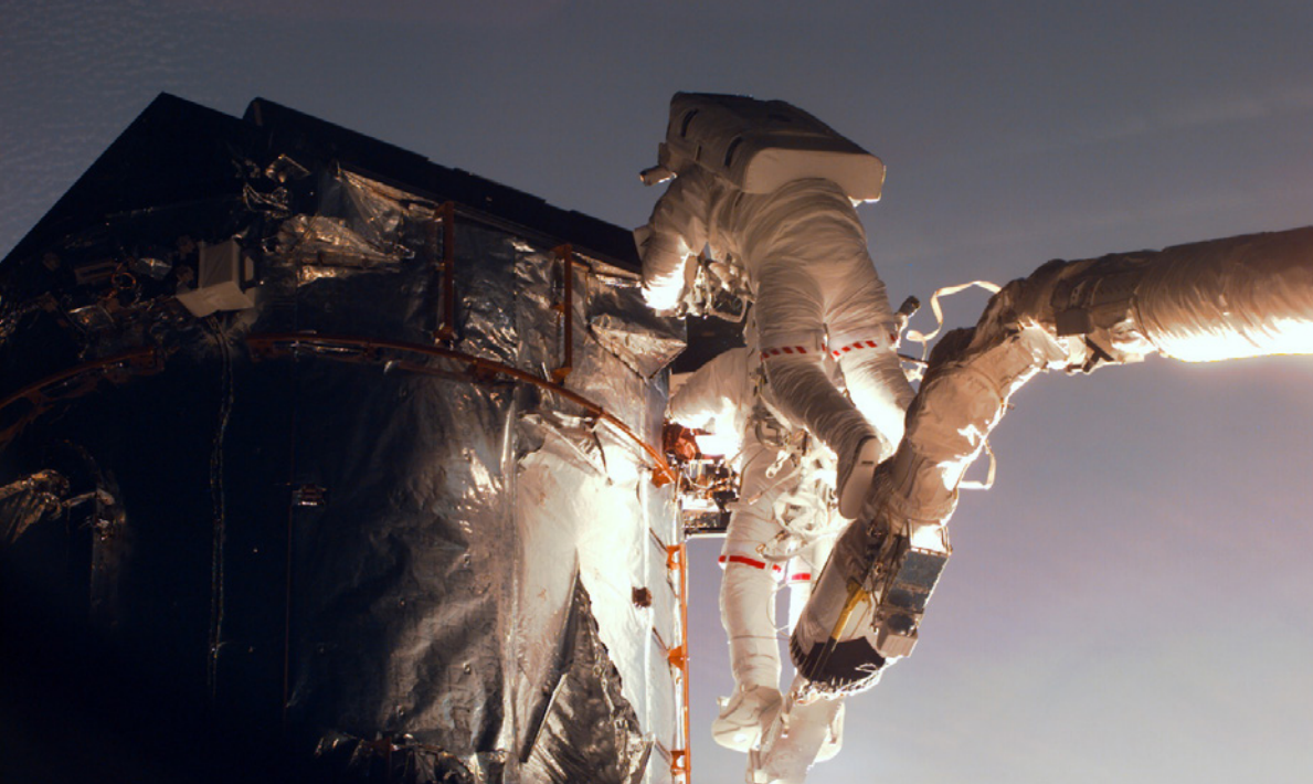
Gregory Harbaugh (solid stripe on EMU) uses the remote manipulator system (RMS) as a cherry-picker device to service Hubble. In cooperation with Joseph Tanner, nearby, Harbaugh is in the process of replacing the Magnetic Sensing System (MSS) protective caps with new, permanent covers. Credit: NASA
