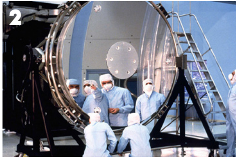
2. Workers study Hubble's main, eight-foot (2.4 m) mirror. Hubble, like all telescopes, plays a kind of pinball game with light to force it to go where scientists need it to go. When light enters Hubble, it reflects off the main mirror and strikes a second, smaller mirror. The light bounces back again, this time through a two-foot (0.6 m) hole in the center of the main mirror, beyond which Hubble's science instruments wait to capture it. In this photo, the hole is covered up.
