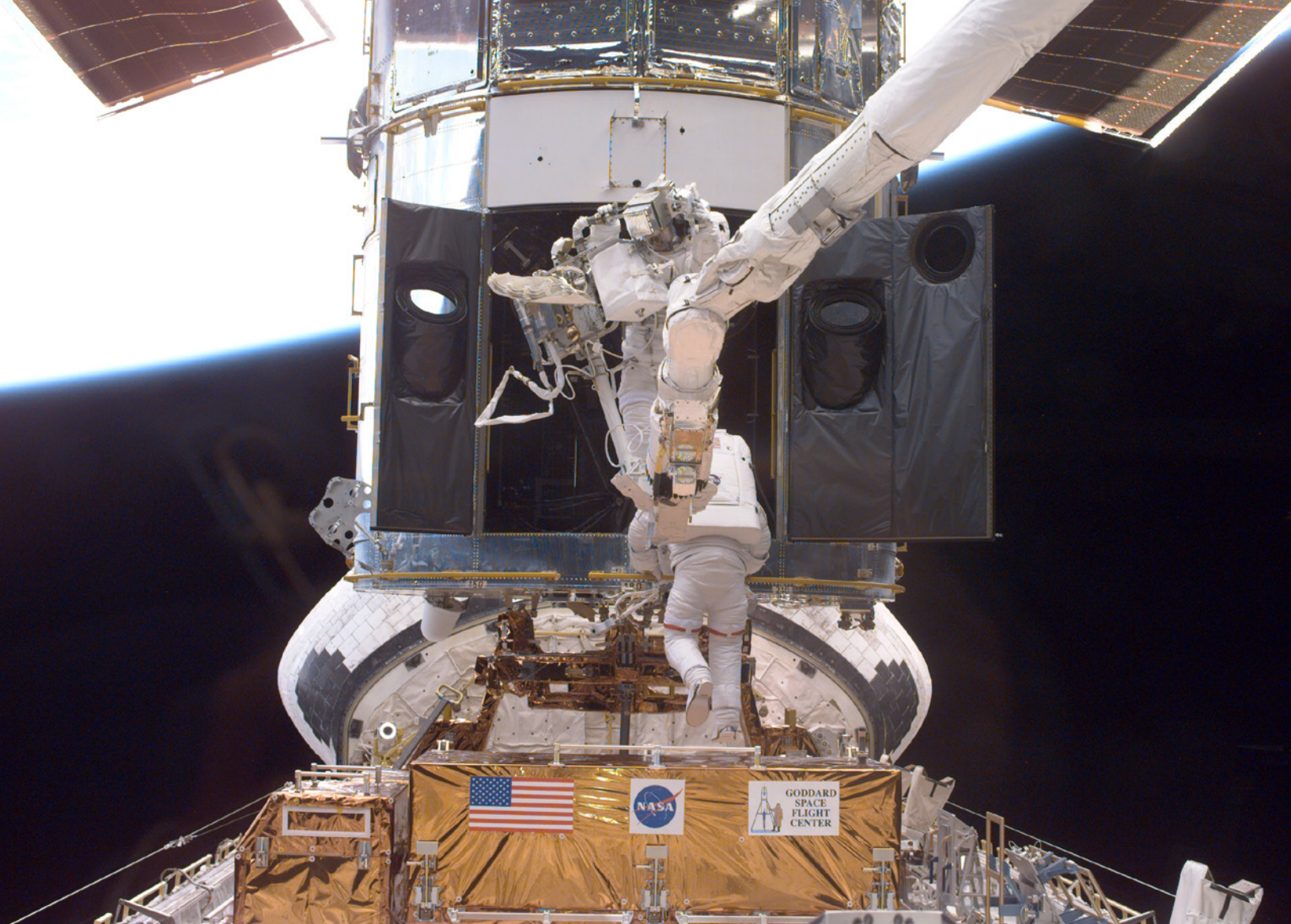
Payload Commander Steven L. Smith (bottom), and Mission Specialist John M. Grunsfeld, perform servicing tasks on the temporarily-captured Hubble Space Telescope. Grunsfeld is on a foot restraint connected to Discovery's RMS robot arm. Smith, making his second servicing visit to HST, is using handrails on the telescope. Credit: NASA
