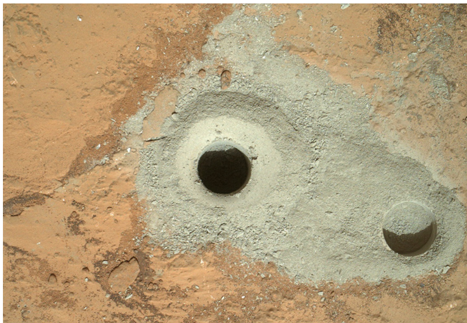
At the center of this image is the hole in a rock where the Curiosity rover conducted its first sample drilling on Mars during its 182nd Martian day of operations. A test that produced the shallower hole two days earlier is shown to the right. The sample-collection hole is 0.63 inch (1.6 centimeters) in diameter and 2.5 inches (6.4 centimeters) deep. The "mini drill" test hole has a depth of 0.8 inch (2 centimeters).
