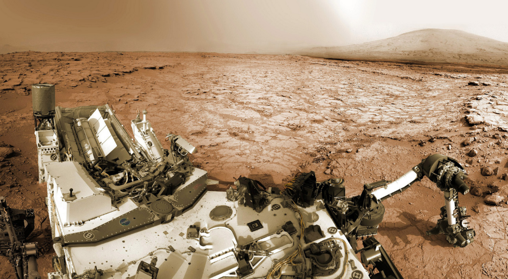
Curiosity is shown in this context mosaic view of the Yellowknife Bay basin taken on Jan. 26 (Sol 169) where the robot is currently working. The robotic arm is pressing down on the surface at John Klein outcrop of veined hydrated minerals – dramatically backdropped with her ultimate destination; Mount Sharp.
